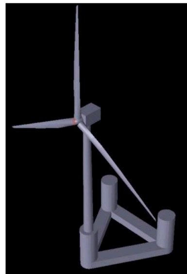
Fig. 2. - The INNWIND semi-submersible three-legged foundation platform [72]. Permission to reuse this figure was given from the EU INNWIND WP4 leader Daniel Kaufer.
