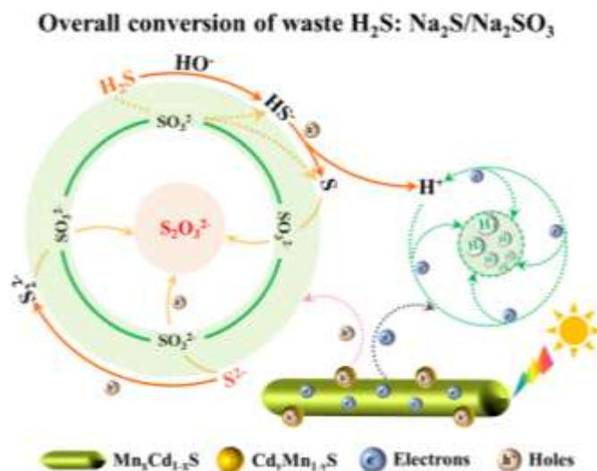
Scheme 1. Illustration of overall conversion of H 2 S and Na 2 S/Na 2 SO 3 over novel Mn x Cd 1-x S/Cd y Mn 1-y S “Dual-Solid-Solution” Z-scheme hybrids.
