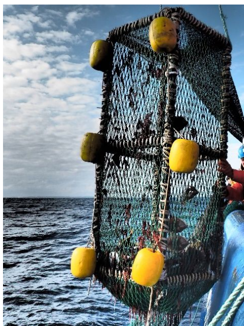
108 Figure 1. Picture of the rigid frame with the fixed meshes (Fixed mesh codend).
