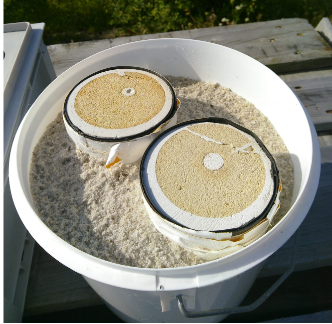
Figure 5.6: Picture of the “calibration” sample, while being exposed to sunlight for 75 days in July-August 2019 at Risø, Denmark. The deepest part of sample 167810, where the luminescence signal was in saturation, is facing upwards.
