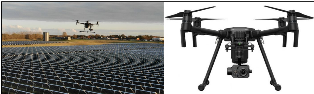
Fig. 1: DJI Matrice 200 equipped with a Zenmuse XT2 camera flying over the solar collector field in Vojens (left) and close-up photo (right) (Drones Made Easy, n.d.).
