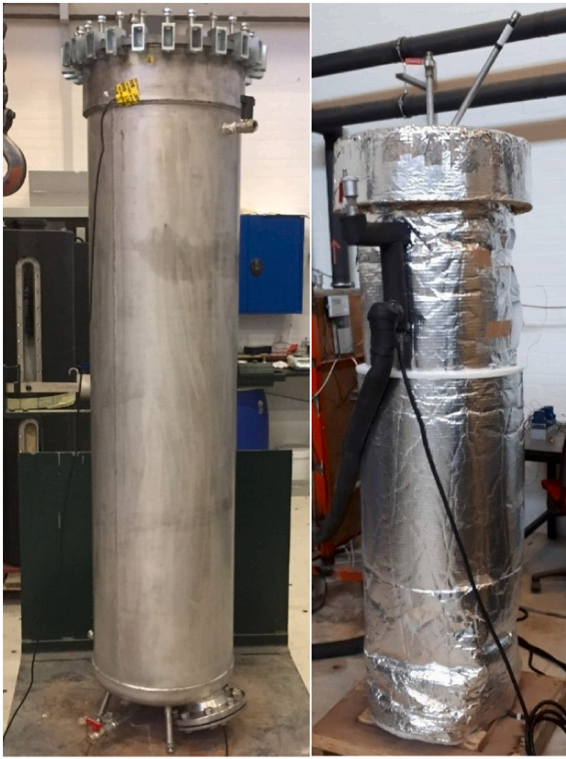
Fig. 5. The PCM water energy storage with (right) and without (left) insulation [34].
