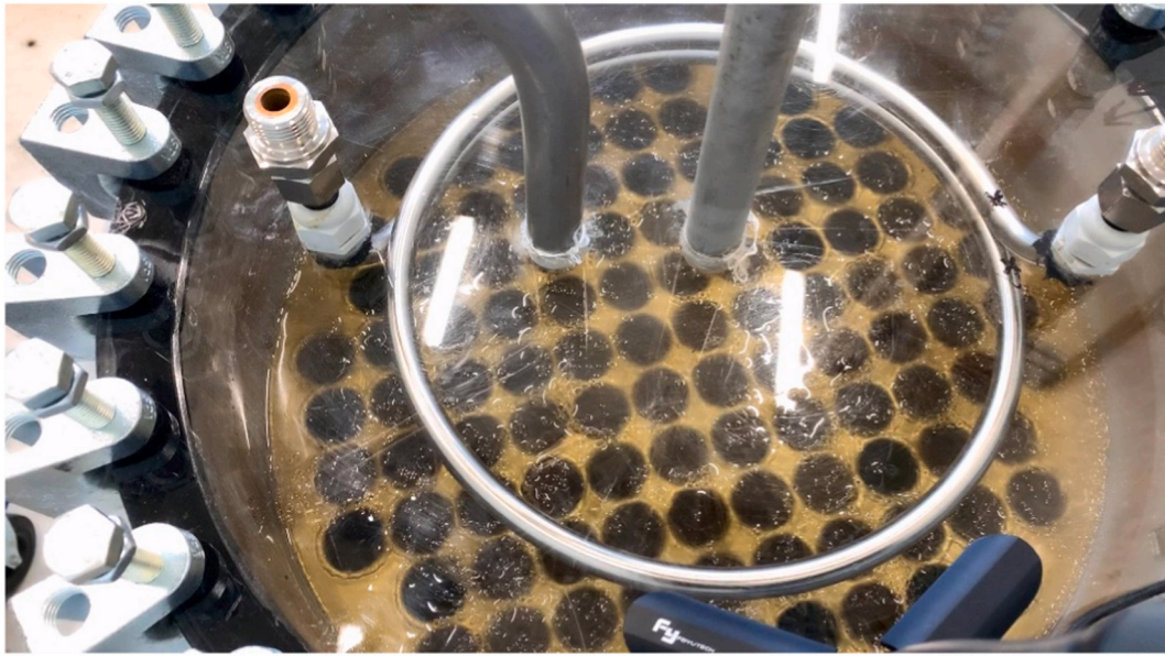
Fig. 7. The manifold plate with a top view of the tubes inside the storage (PCM was melted) [34].
