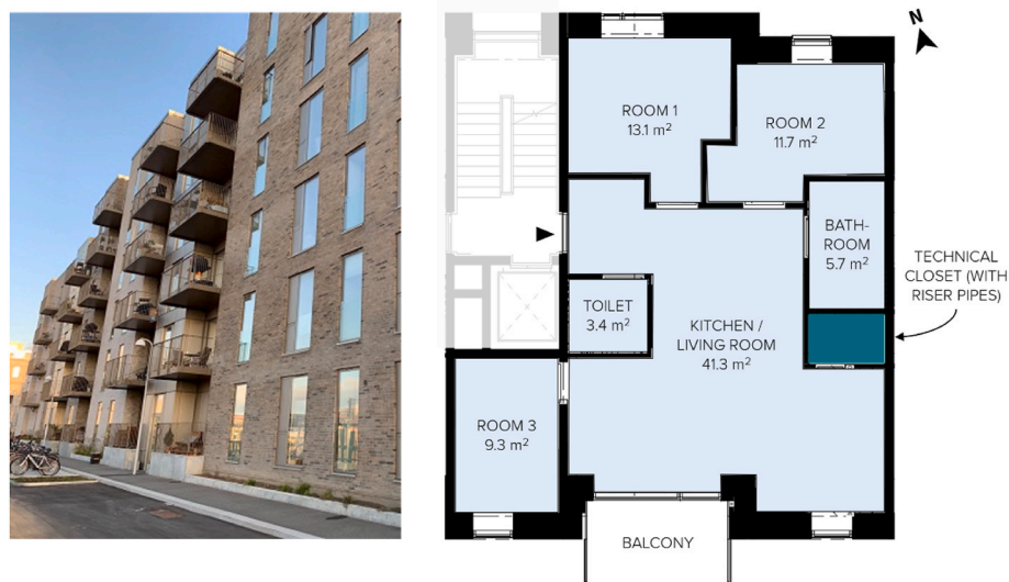
Fig. 2. South-West façade of the building (left, source: [70]) and floor plan of the test apartment (right).
