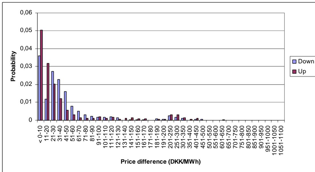
**Figure 6.** Probabilities of regulating up and down for different regulating price intervals, Eastern Denmark, 2002. Observe that the price scale has a finer division for prices less than 200 DKK/MWh.
