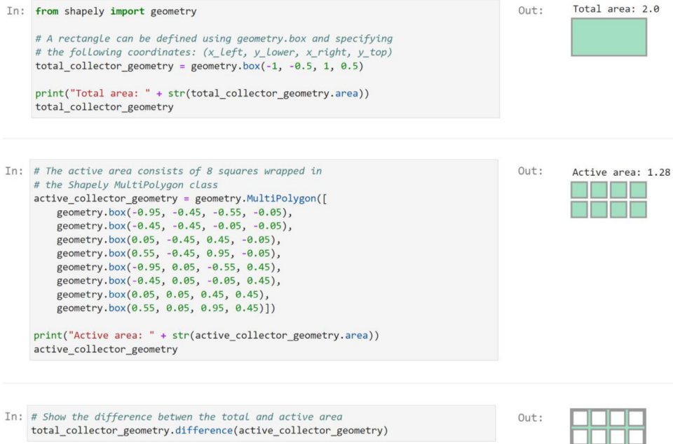
Fig. 2. Example of how to define the total and active collector geometries. The total collector area is represented by a rectangle with an area of 2, whereas the active collector geometry consists of eight squares with a combined area of 1.28.
