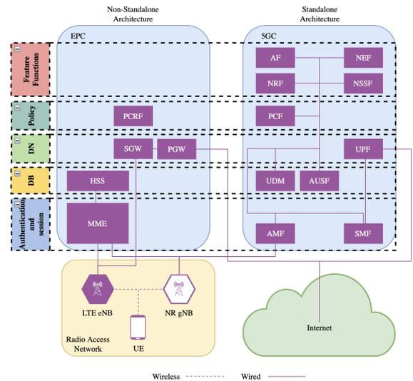
Fig. 2. Comparison of 4G and 5G Core Networks
