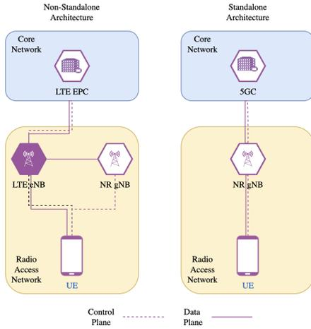
Fig. 1. Comparison of Non-Standalone and Standalone Architecture
