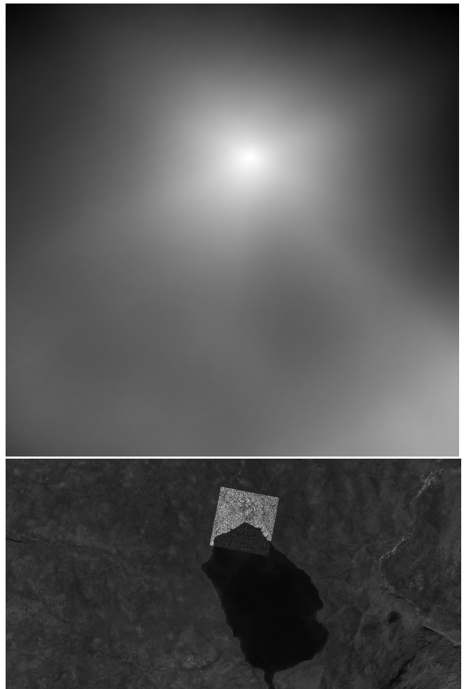
Fig. 6. Mutual information map for radar chip 7 and the resampled SPOT data (top) and best estimated position of chip (bottom).
