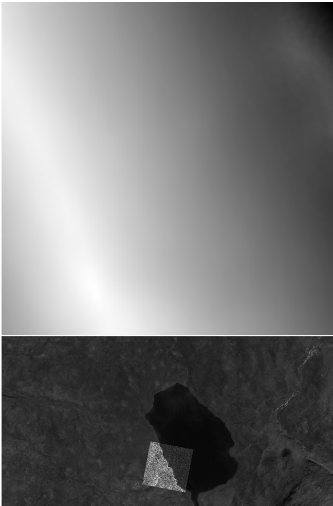
Fig. 7. Correlation map for radar chip 8 and the resampled SPOT data (top) and best estimated position of chip (bottom).
