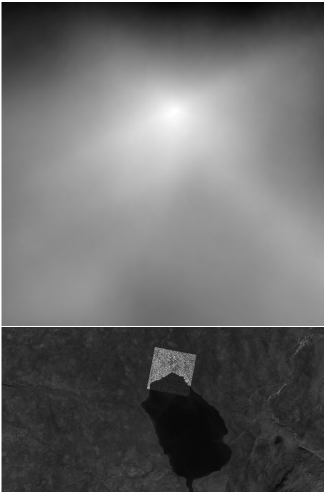
Fig. 5. Correlation map for radar chip 7 and the resampled SPOT data (top) and best estimated position of chip (bottom).
