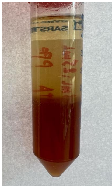
Figure S1. coacervate of PPO-TA obtained after mixing and over-night standing of the PPO (40 wt. %, 25 g) and TA (40 wt. %, 25 g) aqueous solutions
