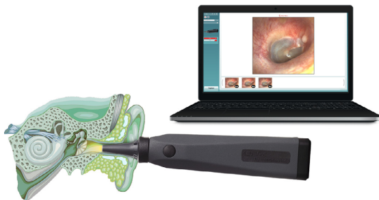
Fig. 2. Sketch of an otoscopic examination with a modern otoscope. The image of the tympanic membrane is shown on an external monitor. Image from Intercoustics A/S.
