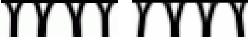
Fig. 2. Optimized bridge topologies for standard compressible elasticity. Left: standard displacement based approach. Right: mixed form approach. The initial and final compliances are W_{init} = 5.244 and W_{final} = 0.788 and W_{init} = 5.245 and W_{final} = 0.806 , for the two cases, respectively.
