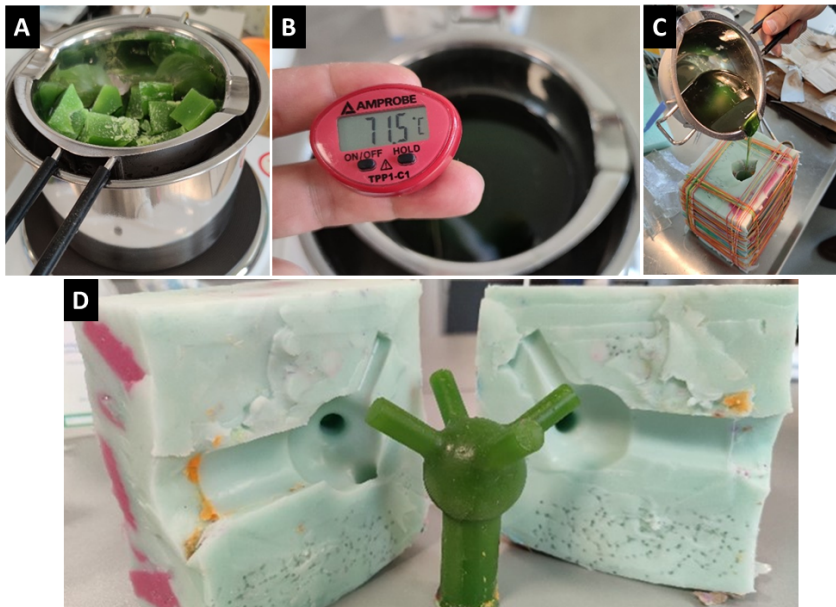
Figure 7.4: The procedure of casting the soluble core is displayed in the figure. A) Melting the solid wax in the melting pot, 2) Monitoring the temperature of the liquefied wax, 3) Pouring liquid wax into the silicone mold, and D) The final solidified water-soluble core.
