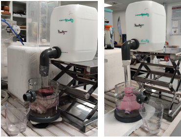
Fig. 4: The expansion experiment setup. The experiment setup consists of a bucket, a Polica 90 degree elbow joint tube, a transparent straight polycarbonate plastic tube, a transparent container and a measuring cup. The left panel shows testing the porcine heart and the right panel displays the test on molded LA chambers.
