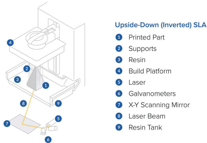
Figure 2.3-3: A graphical representation of the basic mechanics of inverted stereolithography (SLA) printer. 155
