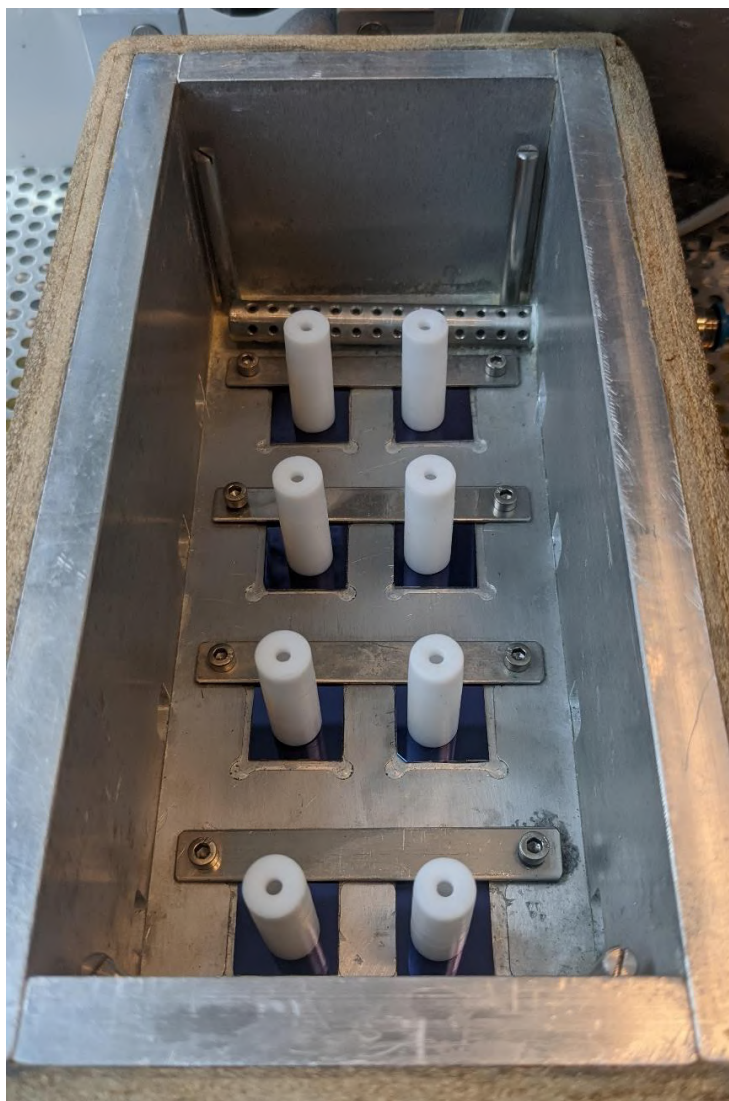
Figure S11: Frozen ice cylinders (in cuvettes) on coatings.
