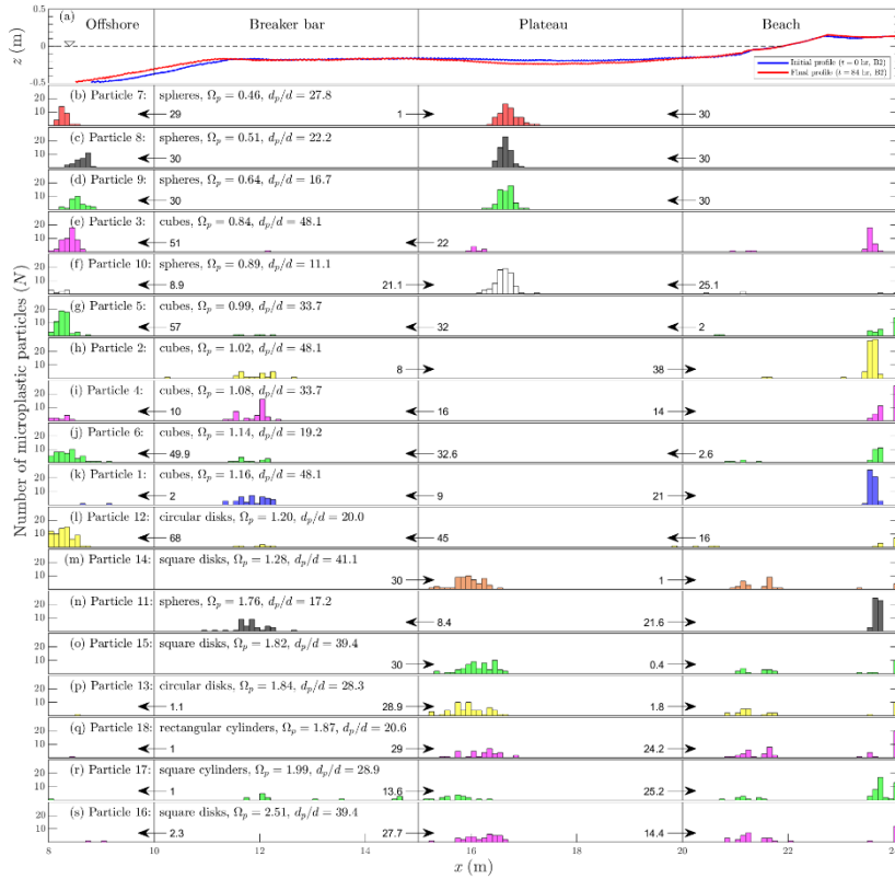
Fig. 2. Plots showing (a) initial (blue line) and final live (red line) sediment bed profiles and (b-s) final cross-shore distribution of microplastic particles, in ascending order based on the particle Dean number \Omega_p . This figure is reproduced from Guler et al. (2022).
