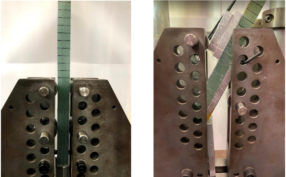
Fig. 3. Picture of the specimen fixture with no initial inclination of the specimen and b) with an initial inclination of the specimen.
