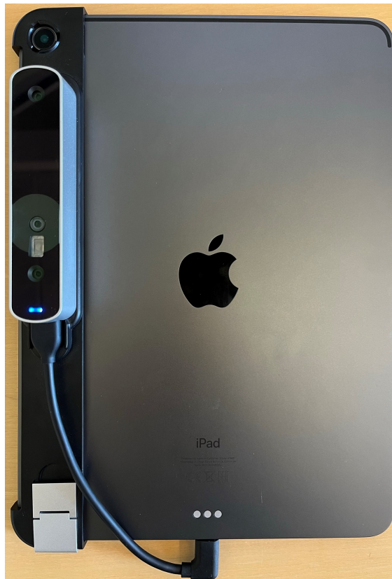
Figure 3.1: A Structure Sensor from Occipital Inc attached to an Ipad Pro from Apple used to capture 3D craniofacial surface scans. Although newer and more expensive versions of the sensor are now available, the cost of the original Structure Sensor used for this study was $379. The Structure Sensor utilizes an infrared sensor to capture objects in 3D and has a depth resolution of 640x480, recommended range of 0.4-3.5 meters, and a field of view of 58x45.
