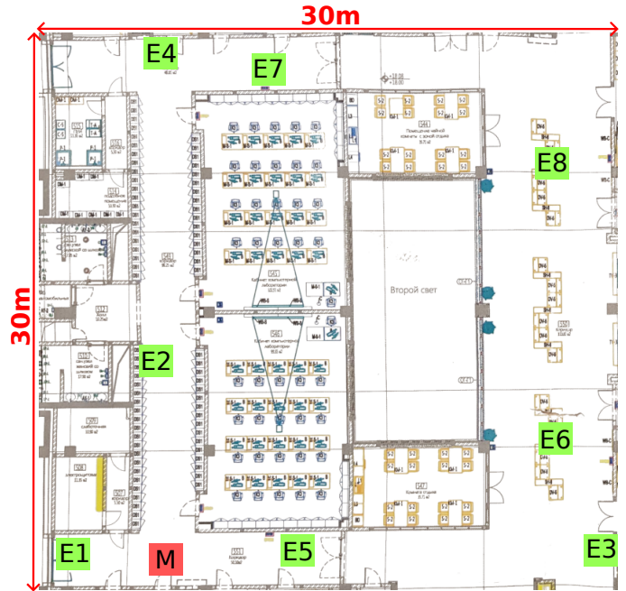
Fig. 8. Locations of the devices during the experiments. [M: transmitter position (master), E1-8: ED positions (slaves)]
