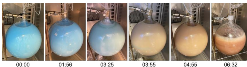
Figure 2.2: Photo series showing the change in colour of batch#1 (5 L, 100 °C) during the reaction. After around 5 h the flask tilted over causing the lower amount of solution seen in the last picture.
