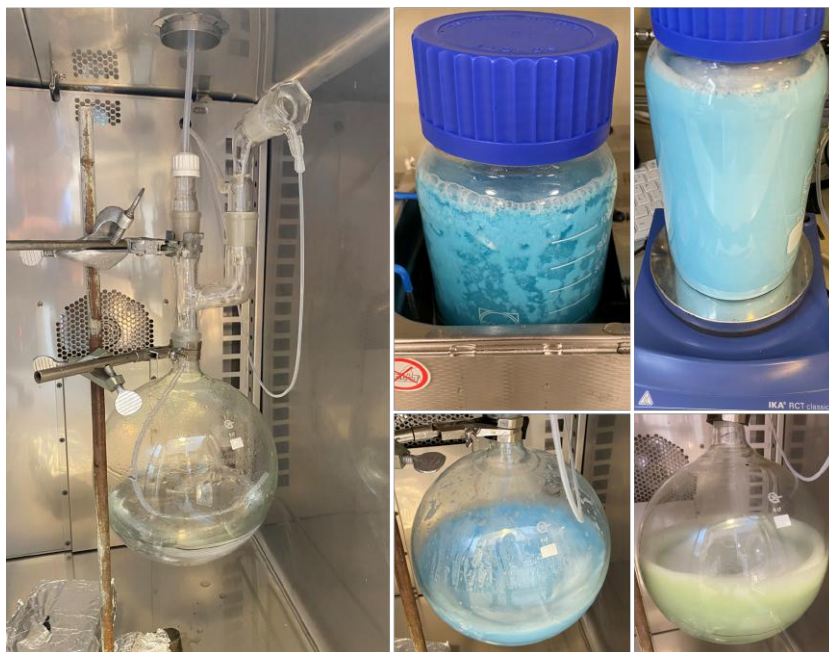
Figure 2.1: Left picture shows the setup in the oven. Upper right pictures show the sonification and stirring of the solution. The lower right pictures show the colour change in the solution during the reaction.
