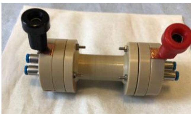
Figure 4.1: Original cell design. The metal inlets in the ends and the electrical connections needed to be redesigned.
