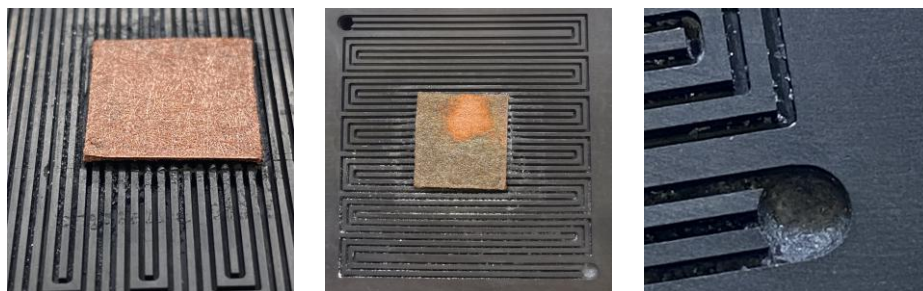
(a) Right after disassembly. (b) After drying in air. (c) The blocked outlet.
