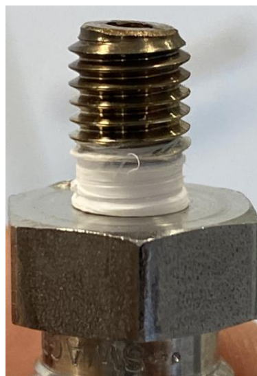
Figure 3.4: Picture of the discoloured Swagelok Part
