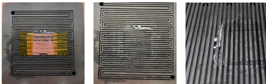
(a) Cathode GDE after the experiment. (b) Salt precipitated above the GDE. (c) Closeup of the salt.
