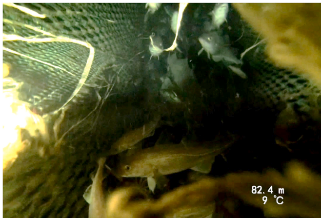
Fig. 3. Video frame of the codend at the beginning of the haul-back phase. The camera was located on the middle of the V-shaped edge of the horizontal panel looking backwards, towards the codline. Haddock were observed in the upper half of the codend whereas cod were seen in the lower half of the codend.
