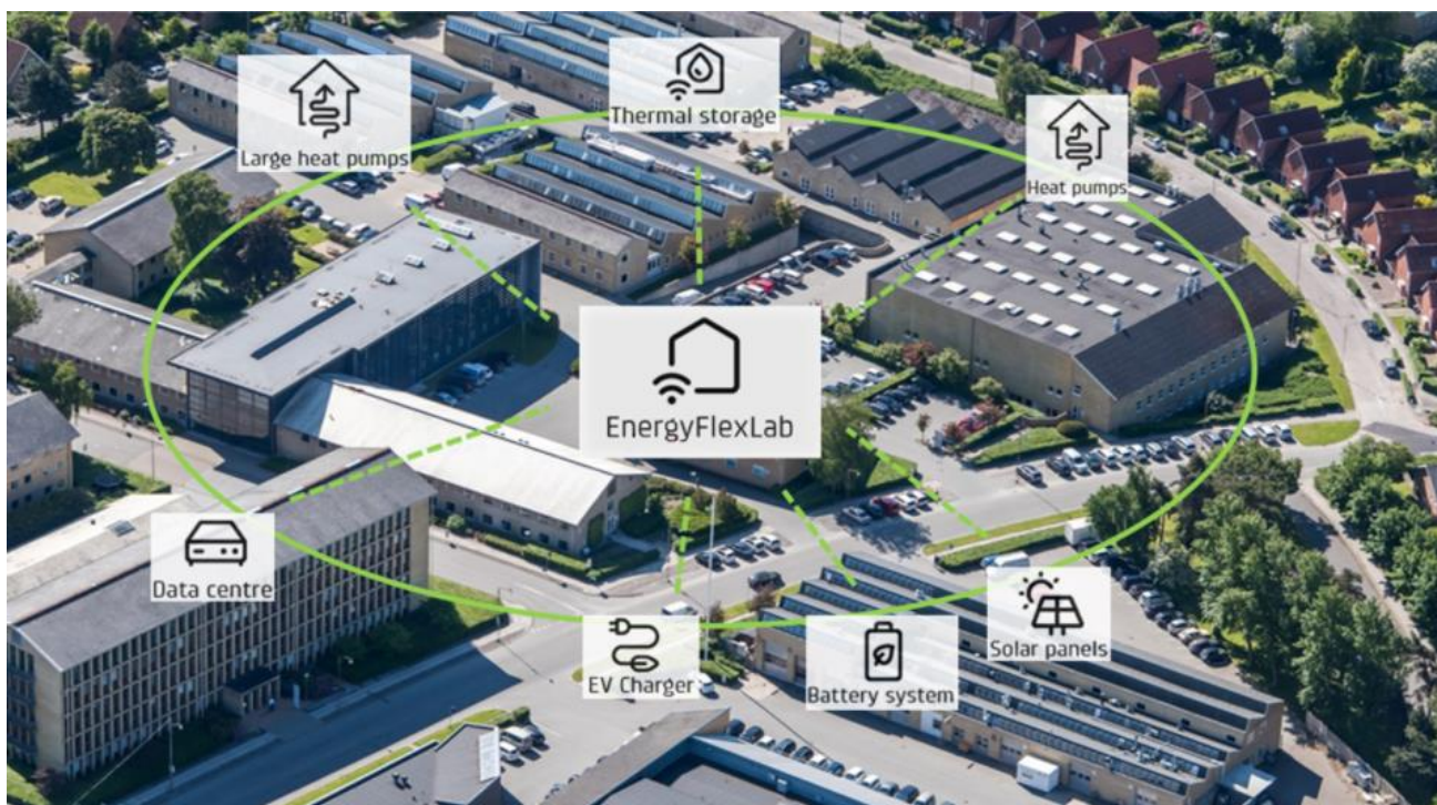
Figure 1: Main components in EnergyFlexLab.
