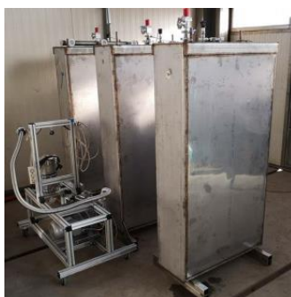
Three prototype modules for a seasonal solar thermal storage system using potassium carbonate as TCM, CREATE project. (Source: AEE INTEC, Austria)
