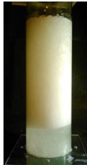
PCM crystallization from supercooled phase – temperatures obtained with a thermal camera (left) in a cylinder with PCM solidifying from top to bottom. (Source: Technical University of Denmark)
