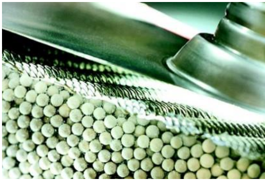
Zeolite beads in the heat exchanger of the zeolite dishwasher. (Source: ZAE Bayern)
