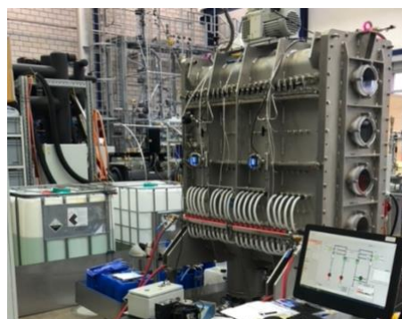
Liquid-sorption-based heat storage system developed at the Lucerne University of Applied Science. (Source: University of Applied Sciences, Lucerne, Switzerland)
