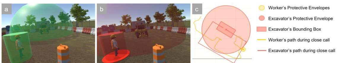
Fig. 1: (a) Worker approaches dozer, (b) close call detected, (c) one buffer event registered, incl. the trajectories of both resources during close call event.
