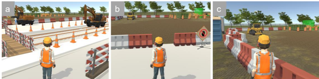
Fig. 10: (a) A secure bridge to the left offers a safe path for crossing the railway under construction, (b) a gap between the barrier may lead a user to enter a restricted work zone, and (c) a safe alternative.
