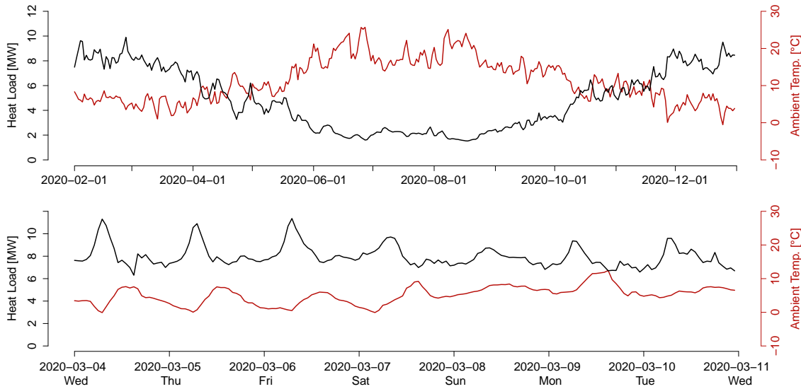
Figure 3.1: The figure shows heat load from one area in Brønderslev. The top plot shows the daily average of the heat load and the ambient temperature over one year, while the lower plot shows the hourly consumption over one week and the ambient temperature.
