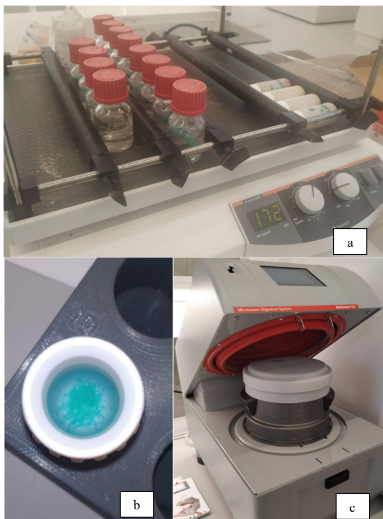
Fig. 11.3 Illustration of the instruments used in obtaining metal adsorption curves. a —fishnet PE in contact with metal solution in a shaking table; b —PE in a Teflon vial in preparation for microwave digestions; c —multiwave GO microwave digestion system. Photograph by the authors
