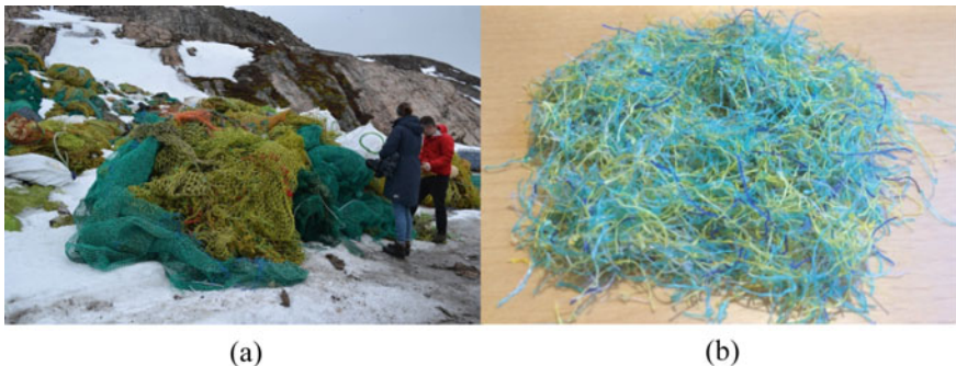
Fig. 12.1 a Discarded fishing nets piled up at the landfill site in Sisimiut, Greenland. b Monofilament R-PE fibers from discarded fishing nets processed by a mechanical cutting operation by the Danish recycling company, Plastix A/S (Bertelsen 2019)
