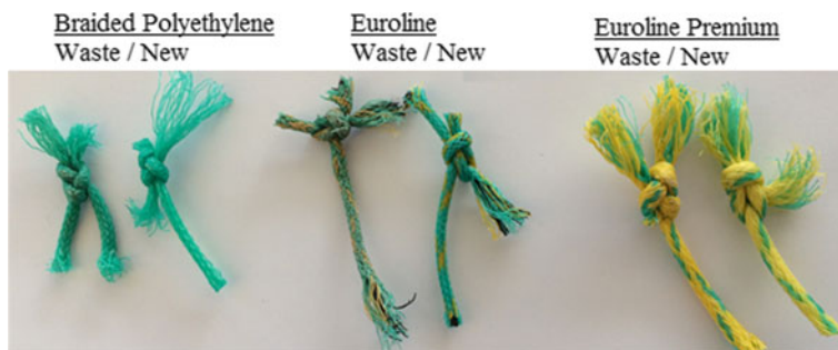
Fig. 12.4 Waste and new PE fishing nets from Euronete, used for characterization of mechanical properties. “Braided Polyethylene” (BP), “Euroline” (EU), and “Euroline Premium” (EP) (Bertelsen and Ottosen 2021)
