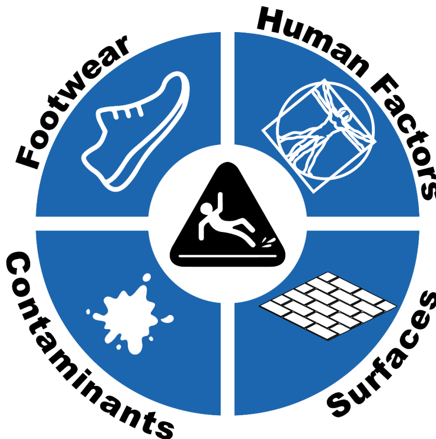
Figure 3 Factors affecting slip resistance.
