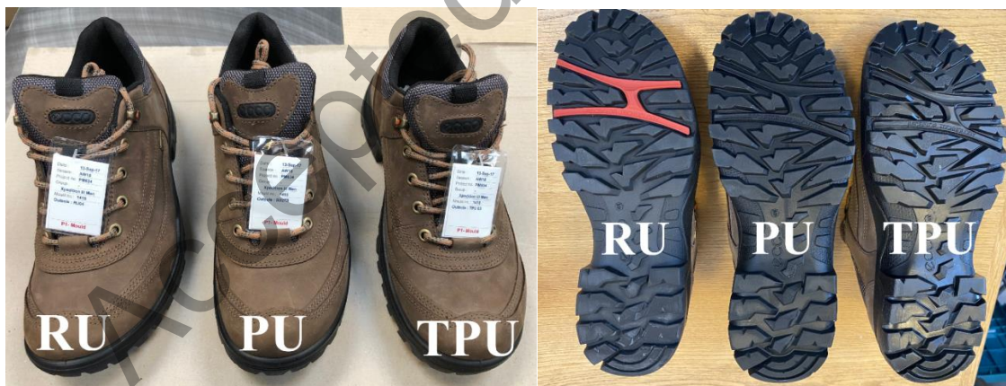
Figure 1: Testing prototypes/shoes constructed of RU (left – note the red part in the forefoot is also RU), PU (middle) and TPU (right).
