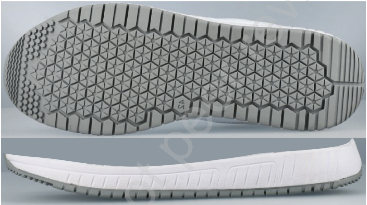
Figure 1. Shoe #1 outsole pattern (top) and profile (bottom).
