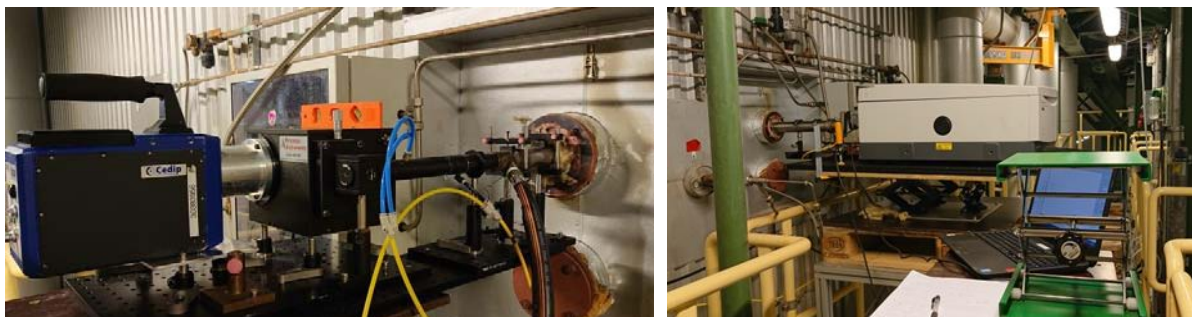
Figure 9. Parallel fast IR emission measurements with IR spectrometer and CEDIP IR camera (left panel: left boiler side) and FTIR spectrometer with sweeping probe (right panel: right boiler side). Both systems are viewing the same axis.
