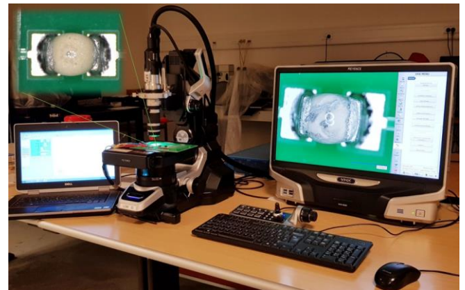
Fig. 2. Droplet test on an SMC in connects to potentiostat under a digital microscope.
