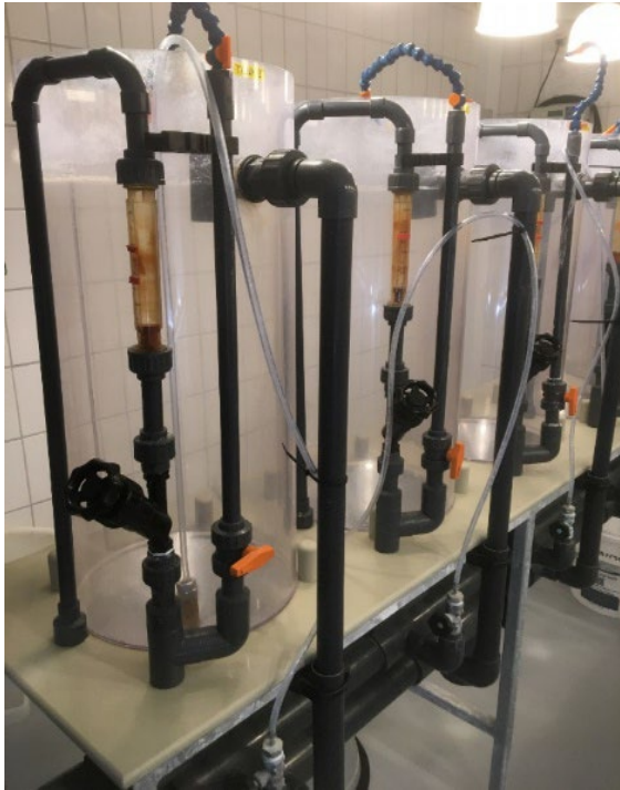
Figure 10. Experimental up-flow 50 L tank at DTU Aqua for research.
