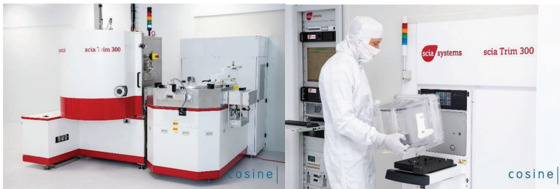
Figure 6: Ion Beam Figuring machine (left) including a fully automated wafer cassette loader (right), as recently installed at cosine.
