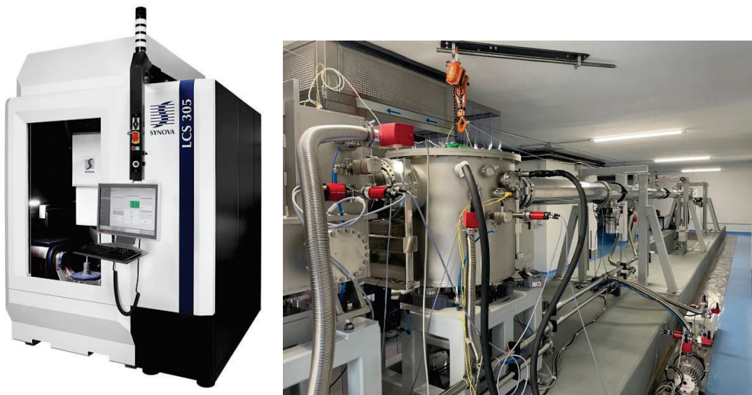
Figure 8: Laser computer numerical controlled (CNC) machine to cut oversized stacks to size (left). BEATRIX beamline, as installed at BRERA (right).
