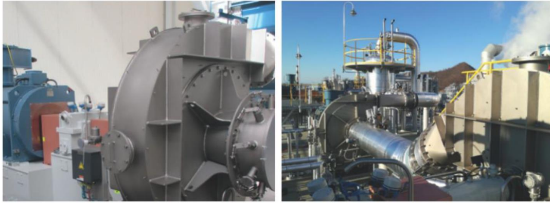
Figure 2-7: left - PILLER High Performance Blower, right - multi-stage system in operation.
