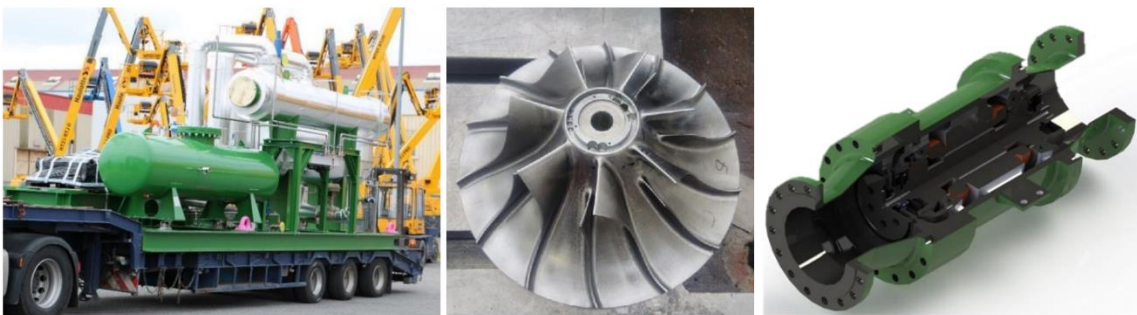
Figure 2-2 Example of Enertime Heat Pump with a capacity of 3.7 MW.
