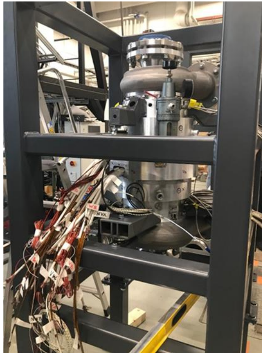
Figure 4-15: Developed bearingless high pressure ratio heat pump compressor.
