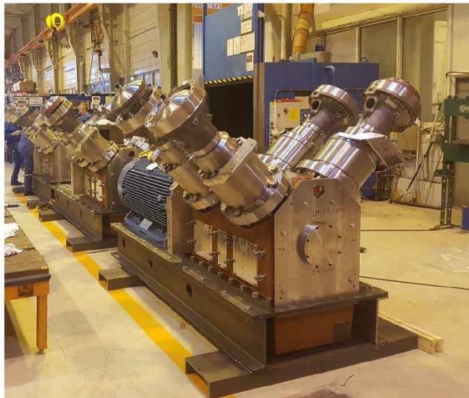
Figure 2-27: Production of the HighLift high temperature heat pump at Olvondo.
