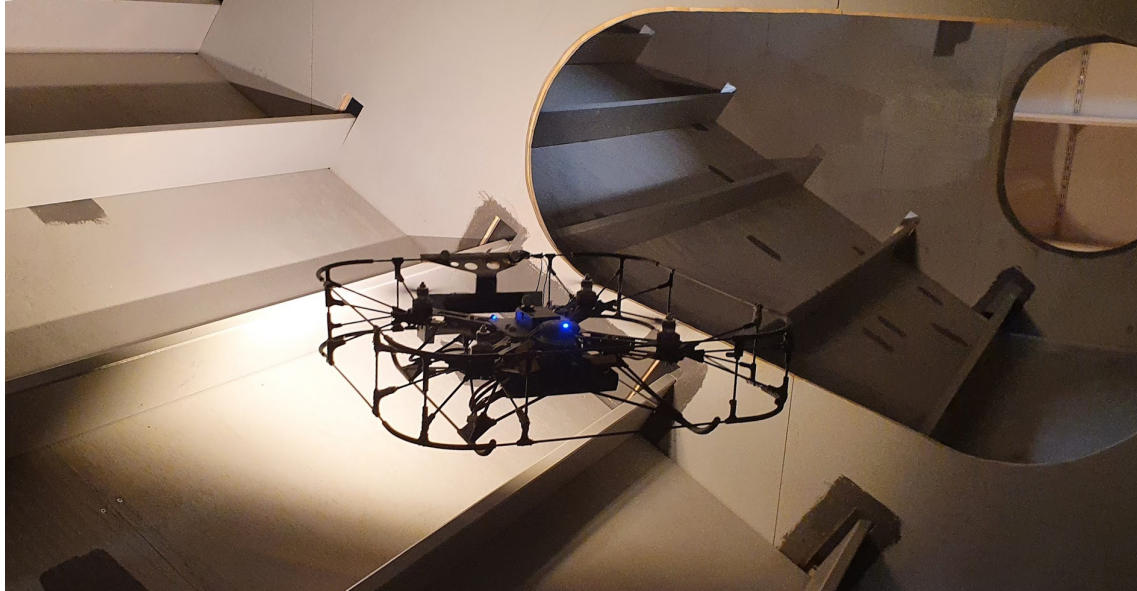
Figure A.3. Example of a drone flying in a ballast tank. If equipped with the right sensory equipment accompanied by a high level of autonomy, the drone can replace human surveyors in the hazardous environments present in the ballast tanks of modern marine vessels.
