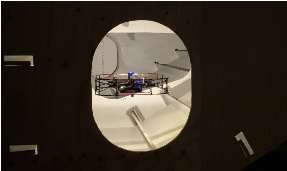
Figure B.1. Our system operating inside the mock-up ballast tank, in complete darkness.
