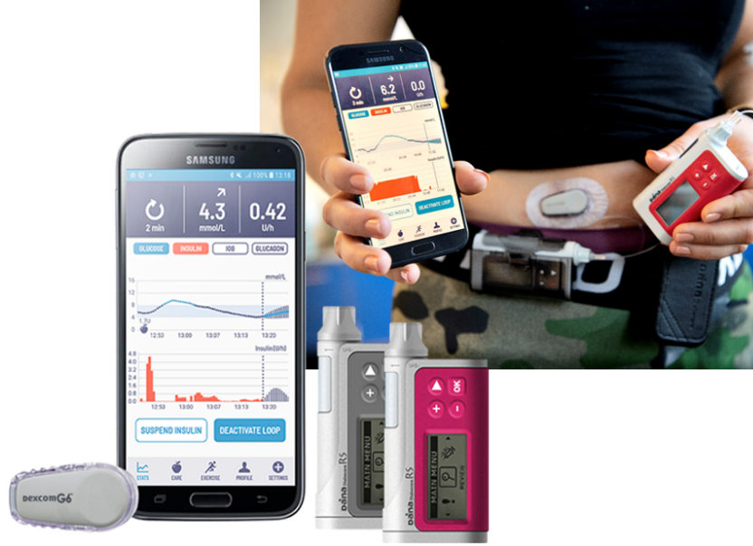
Figure 4.3: The DiaCon AP system. The system consists of 1) an Android smartphone, 2) a Dexcom G6 sensor, 3) a Dana Diabecare RS pump for insulin administration, and 4) another Dana Diabecare RS pump for glucagon administration.
