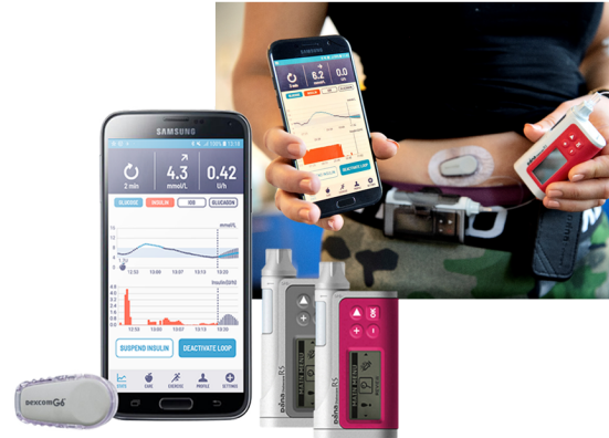
Figure 1: The DiaCon AP system. The system consists of 1) an Android smartphone, 2) a Dexcom G6 sensor, 4) a Dana Diabcare RS pump for insulin administration, and 5) another Dana Diabcare RS pump for glucagon administration.
