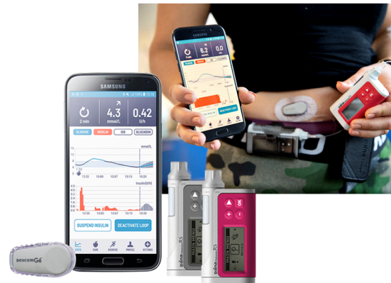
Figure 1: The DiaCon AP system. The system consists of 1) an Android smartphone, 2) a Dexcom G6 sensor, 4) a Dana Diabecare RS pump for insulin administration, and 5) another Dana Diabecare RS pump for glucagon administration.
