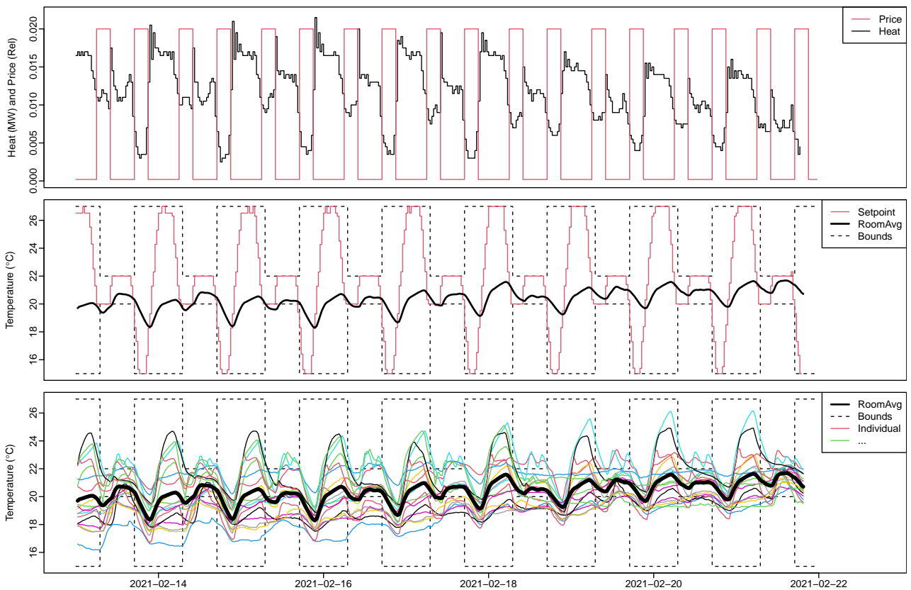
Figure 3: Results from the period running with the tuned MPC. Upper plot is of the price and heat demand. Mid plot is of the temperatures considered by the MPC. Lower plot is of the individual room temperatures and the mean temperature. The latter plots also contain the temperature constraints.
