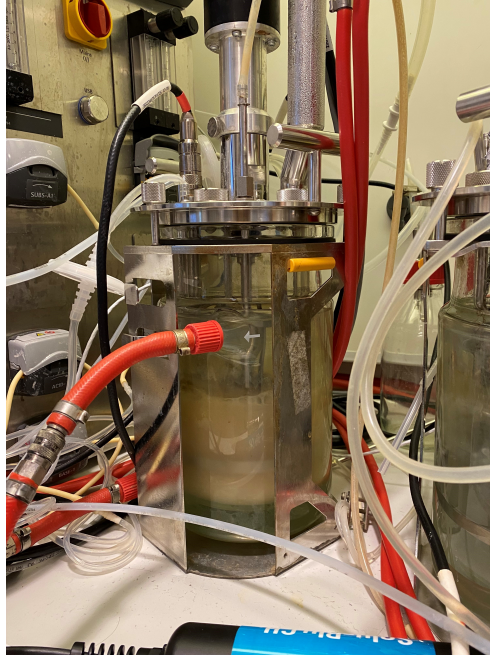
Figure 11.1: Image of laboratory-scale fermenter for single-cell protein production.
