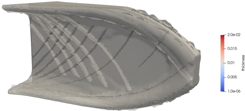
Figure 6.7: Initial dehomogenized cantilever beam. Meshed with 190.000 elements and uniform thickness of 0.01. Part of the structure has been made transparent to reveal the internal stiffeners. The initial compliance is \mathcal{C} = 0.170 \text{ J} ( \mathcal{C}_m = 0.163 \text{ J} , \mathcal{C}_b = 0.007 \text{ J} ), and the initial volume is 0.144 \text{ m}^3 .
