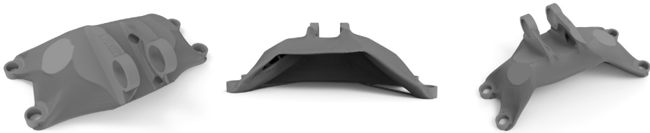
Fig. 15. Reference design of the bracket example with Robust formulation and consistent boundary condition for PDE-filter. C = 4.21 \times 10^7 J.
