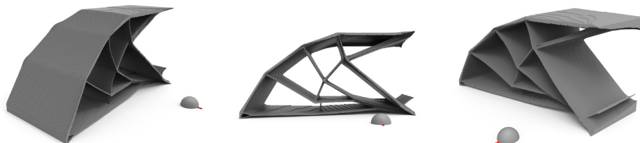
Fig. 10. Cantilever beam with a single milling direction from the side. C = 1.37 \times 10^7 .
