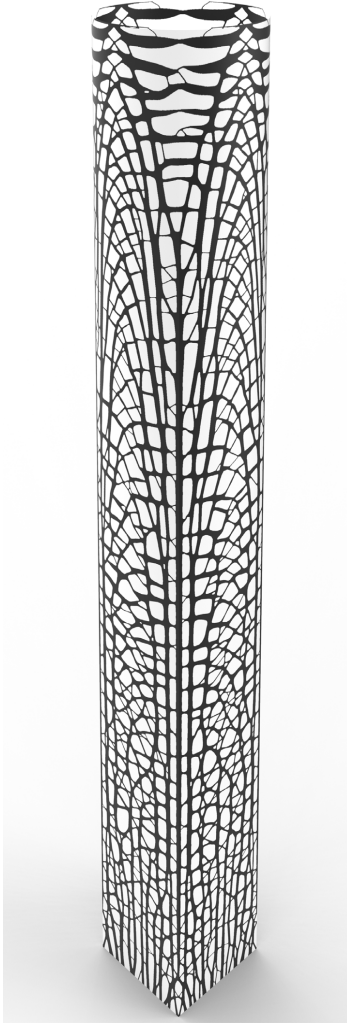
Fig. 11. Resulting topology of the Lotte tower example with filter radii of r_{\text{solid}} = 22.5 cm and r_{\text{LV}} = 4.5 m.
