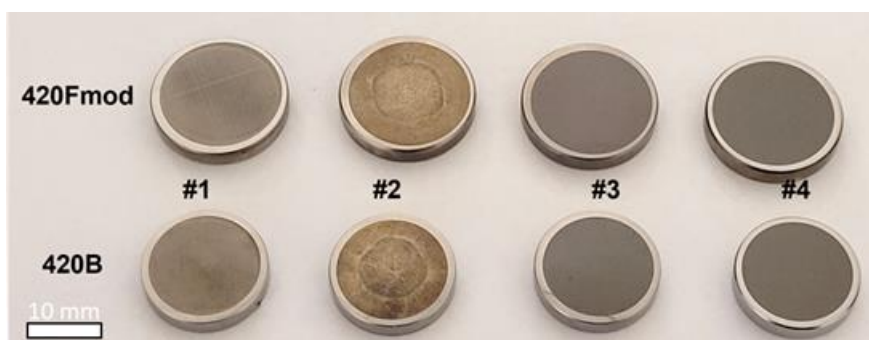
Figure. 3.3. Appearance of laser marked samples for both investigated steels, for all four laser marking parameter sets
