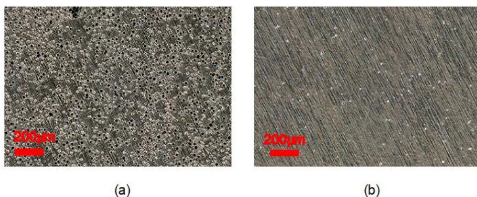
Figure 4.1: LOM micrographs of laser marked surfaces of nitrided samples of (a) 1.4197 and (b) 1.4028.
