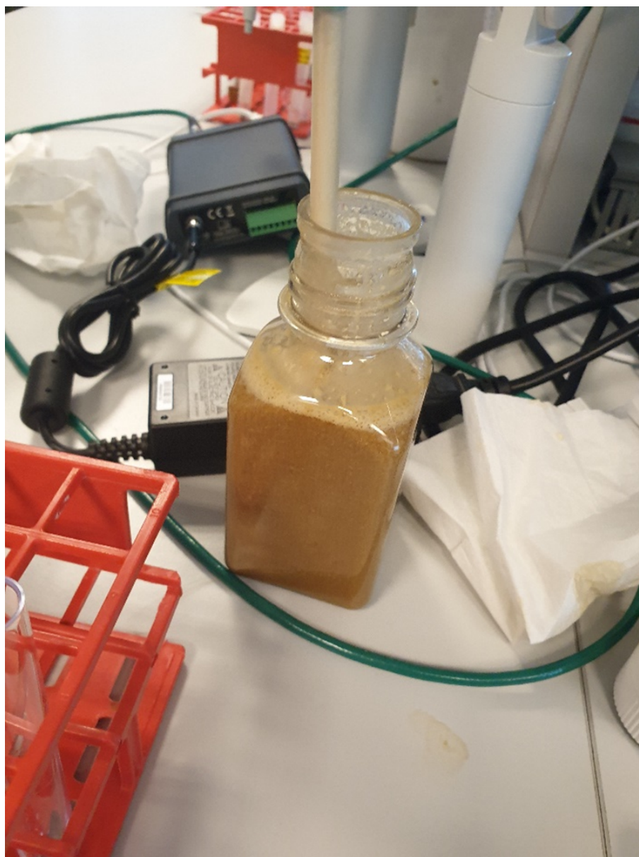
Figure A.4: Dielectric spectroscopy reading of approximately 100 mL bulk sample with the ABER FUTURA Pico probe
