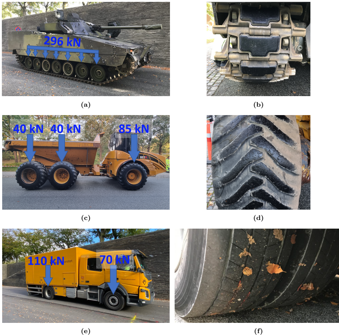
Figure A.8: Test vehicles: (a) military tank, (b) military tank track, (c) dumper truck, (d) dumper truck tires, (e) VIAFRIK, and (f) VIAFRIK tires.
