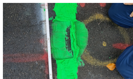
Figure A.9: Imprint from the military tank rubber pads using modeling clay.
