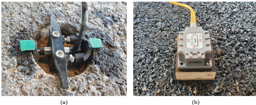
Figure A.12: Surface sensors: (a) LVDT in blind-hole, and (b) tiltmeter.
