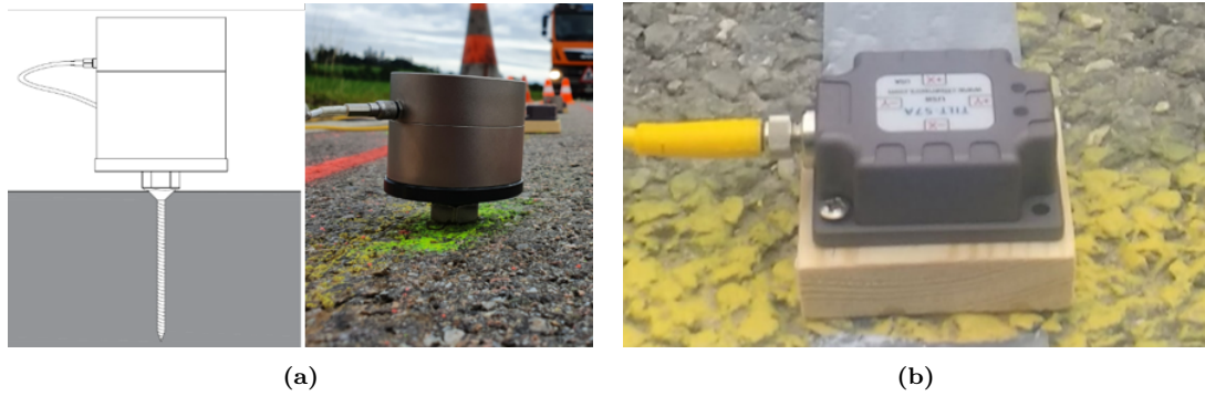
Figure A.16: Surface sensors in La Ferrière: (a) accelerometer and (b) tiltmeter.
