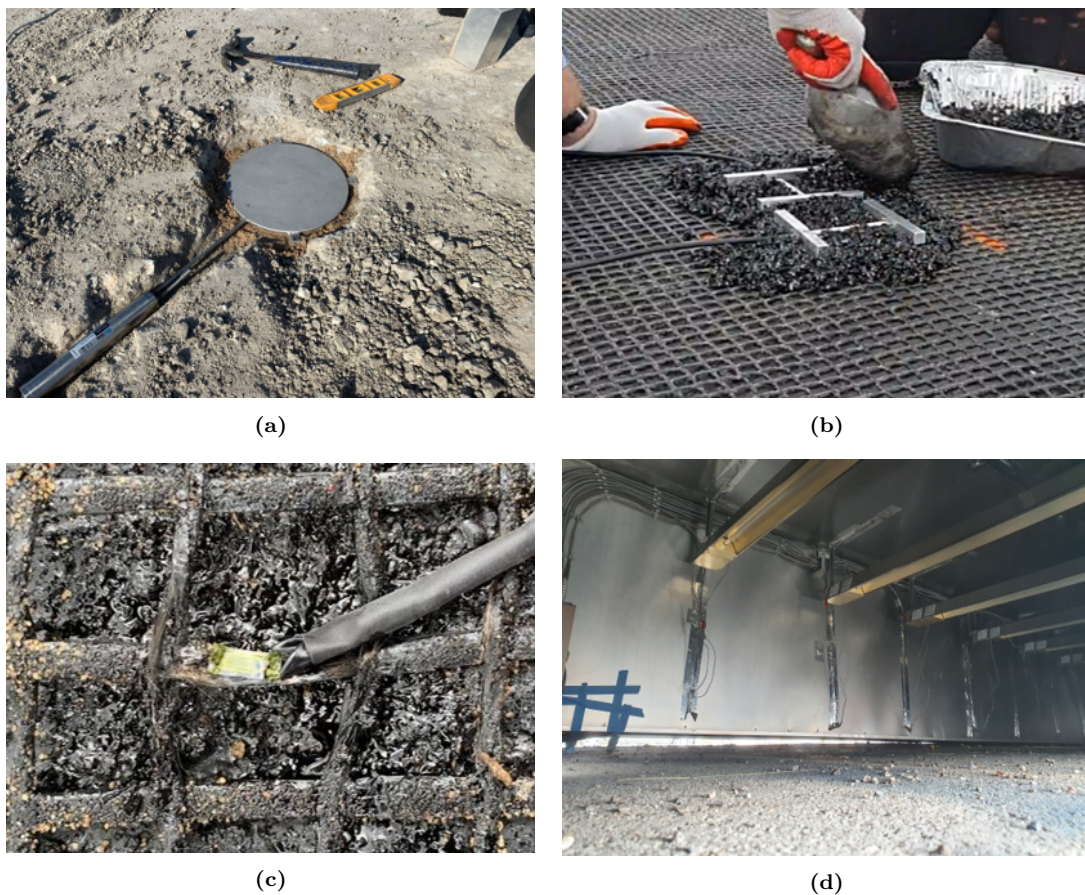
Figure A.11: Pictures from the APT test setup at UTA: (a) pressure cell, (b) ASG, (c) grid gauge, and (d) aging box (inside).
