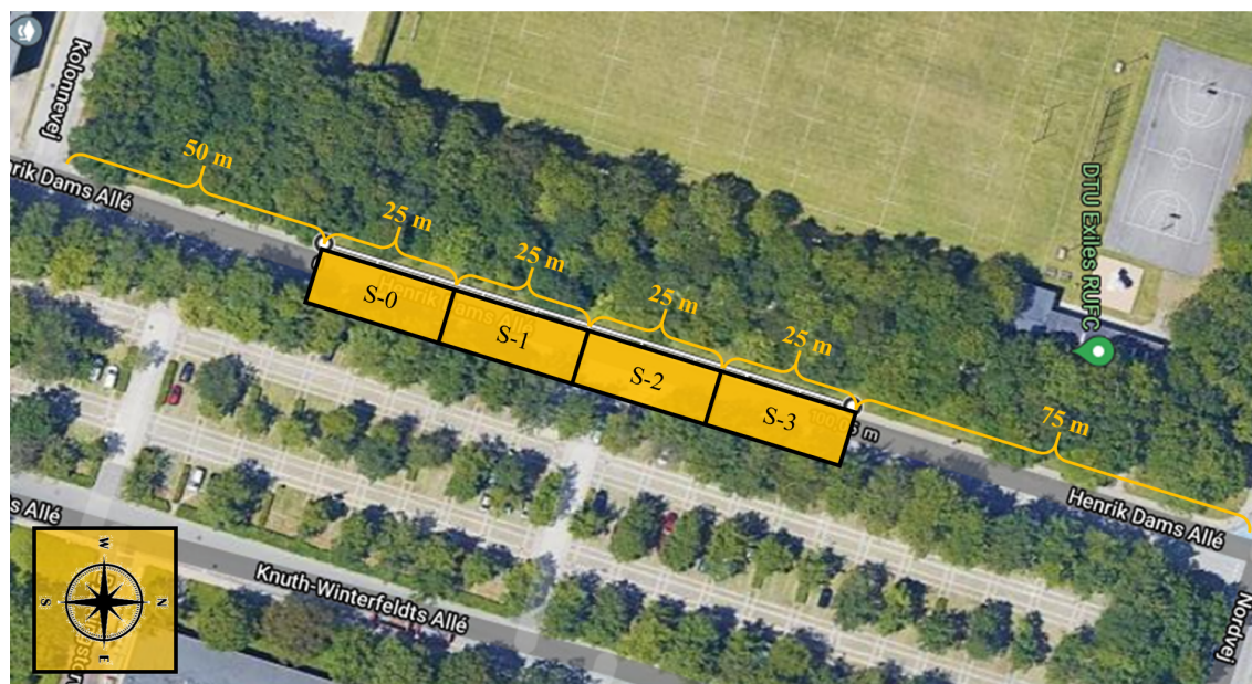
Figure 3.15: DTU Smart Road: Overview of the four test sections.
