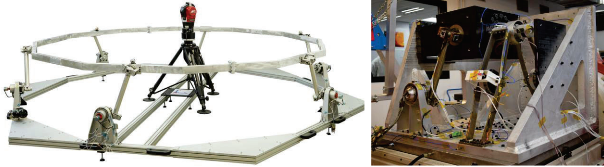
Figure 4: (Left) Test configuration of the ISM hexapod configuration developed by SENER Poland used to verify the required positioning accuracy performance. A dummy is used for representing the inertia of the MS. This concept demonstrated all the requirements in terms of accuracy and stability (around 10 \mu\text{m} over 1 day). (Right) Test configuration of 1 launch lock and 1 ISM actuator, used to verify the structural integrity, damping and shock from the release as a standalone item. The full verification will be completed once the MAMD environmental tests are completed (where the 6 launch lock systems are included).
