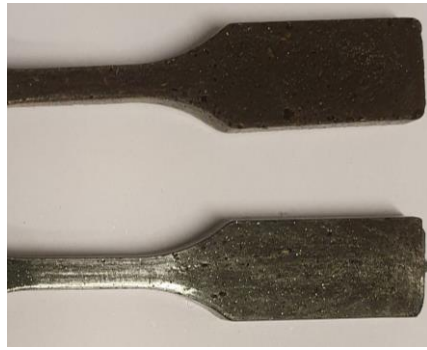
Figure 2 PLA molds with 30% alfalfa pulp (top) and 10% alfalfa pulp (bottom)
