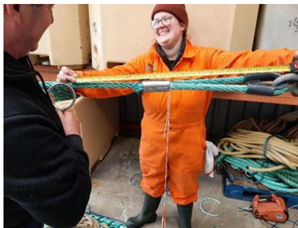
Fig 2.3.3 Mounting upper wing along the headline leading to a 0.74m difference. Note small electric winch on the floor to the right required subsequently to mount the upper wing tips.
