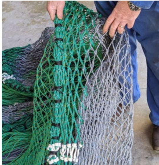
Fig 2.3.2 Heavy double twine guard mesh running along the selvedge.
