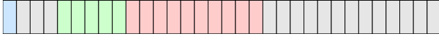
Fig. 1. Alignment of TFP32 numbers in 32-bit words: binary16 ( f=10 , e=5 ) case. Biasad exponents (green) are sign-extended to 8 bits. Significands (red) are padded with zeros beyond bit of weight 2^{-f} .
