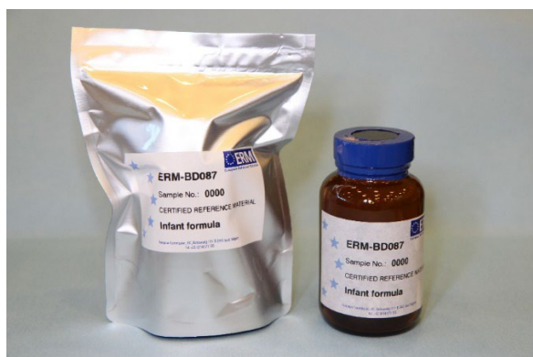
Figure 1. ERM-BD087. Final containment in sachet (left) containing a 100-ml glass bottle (right).
