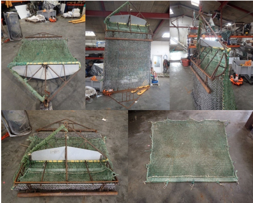
Figure A7.1. The mussel dredge used for the cockle fishing efficiency calibration. The inner net is on the lower right image. Photos P. Freitas.
