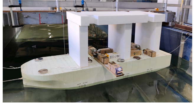
Fig. 2. Ship model of Wind Orca , launched into the basin, loaded to max draught.
